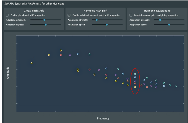
Figure 6.12: Screenshot of SWARM . The user interface shows three adaptation modes: Global Pitch Shift : F0 adaptation as described in Chapter 5, Harmonic Pitch Shift : Using gradients of SD w.r.t. the frequency of individual partials, and Harmonic Reweighting : Using gradients of SD w.r.t. the amplitude of individual partials (while also ensuring that overall loudness is preserved). The bottom plot shows all harmonics that are active in the current frame in real time. As an example, the harmonics in the red circle coincide almost exactly in frequency due to the Harmonic Pitch Shift .
