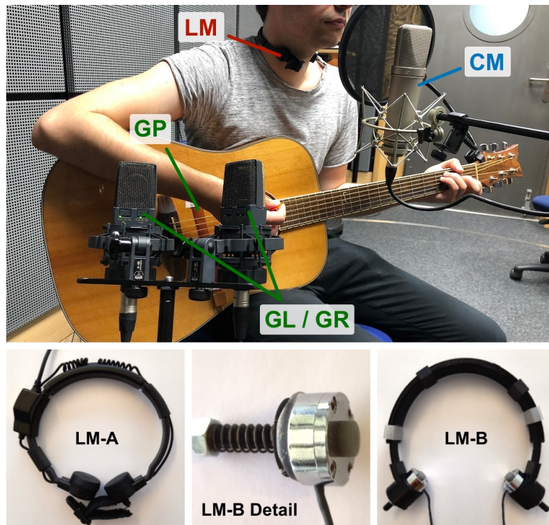
Figure 4.2: Photograph of the recording setup (top) and detailed depiction of the used LMs (bottom). LM-A: Albrecht AE-38-S2a larynx microphone, LM-B: Self-made larynx microphone with TE Connectivity CM-01B sensor, CM: Close-up microphone (Neumann U87), GP: Guitar Pickup (AMG Electronics C-Ducer), GL/GR: Guitar Stereo Left/Right (AKG C414).
